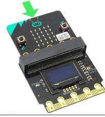
The BBC micro:bit is inserted into the top edge connector. No soldering or tools are required.
