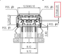
3. The gap increasing between shell and PCB is to avoid short circuit and raise safety factor, and stand-off area change of housing is to avoid soldering overlapping.
