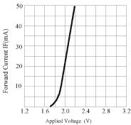
FORWARD CURRENT VS.APPLIED VOLTAGE
