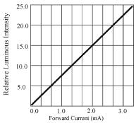
FORWARD CURRENT VS. LUMINOUS INTENSITY
