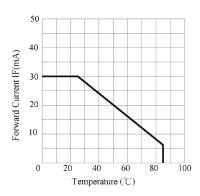
FORWARD CURRENT VS. AMBIENT TEMPERATURE
