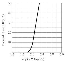
FORWARD CURRENT VS.APPLIED VOLTAGE
