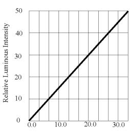
FORWARD CURRENT VS. LUMINOUS INTENSITY
