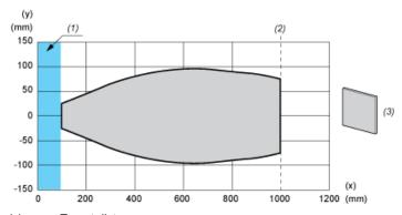
(x) Target distance(y) Detection limit(1): Blind zone: 105 mm
