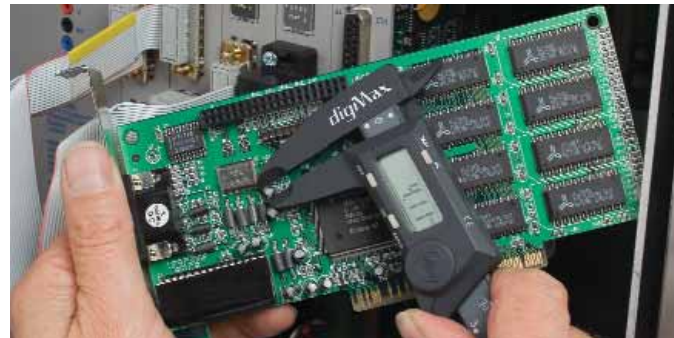
The digiMax calliper can be used for measuring delicate electronic components.
