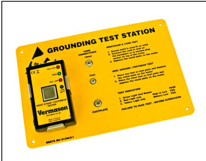
Figure 1. [222506](#) Wrist Strap Test Station.
