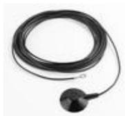
**Ground Cord, 15 ft. (4.6 m), with 10 mm snap. Molded-in male snap fastener with integral 1 megohm resistor on one end, solderless terminal on other. Connects all 3M® Static Control Mats and Runners to building ground.**
