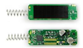
Power is provided to STM 350 by means of a small pre-installed solar cell which works in conjunction with an integrated energy storage element in order to ensure operation in periods without ambient light.
