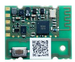
PTM 535BZ provides direct mechanical connection to the ECO 200 harvester by means of 2 contact pads on the PCB. Additionally, PTM 535BZ provides a 5-pin solderable interface for the connection of the ECO 200 harvester together with 2 additional input signals.
