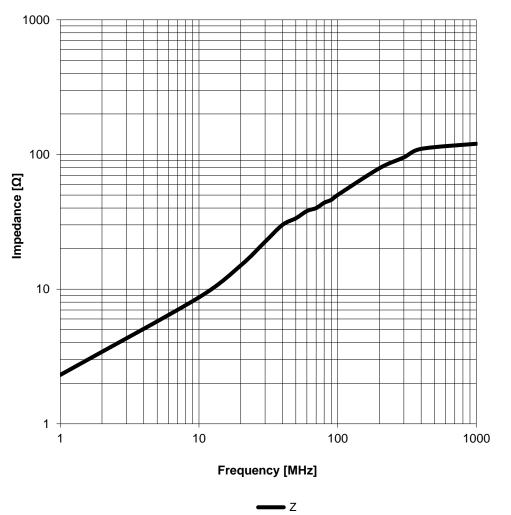
CHECKED REVISION DATE (YYYY-MM-DD) GENERAL TOLERANCE PROJECTION METHOD AlMo 004.006 2018-04-18 DIN ISO 2768-1m **WE-FLAT Flat Ferrite Core** Würth Elektronik eiSos GmbH & Co. KG WüRTH ORDER CODE EMC & Inductive Solutions Max-Eyth-Str. 1 ELEKTRONIK 7427809 74638 Waldenburg Germany STATUS Tel. +49 (0) 79 42 945 - 0 BUSINESS UNIT PAGE YOU EXPECT www.we-online.com 2/4 eiSos Valid eiSos@we-online.com
