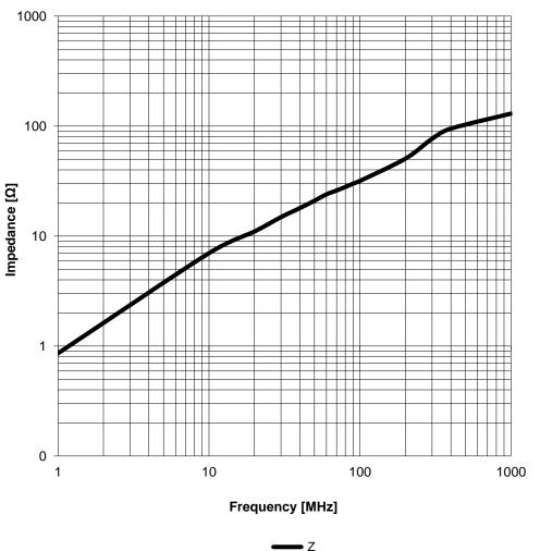
CHECKED REVISION DATE (YYYY-MM-DD) GENERAL TOLERANCE PROJECTION METHOD AlMo 005.000 2018-08-01 DIN ISO 2768-1m **WE-FLAT Flat Ferrite Core** Würth Elektronik eiSos GmbH & Co. KG WüRTH ORDER CODE EMC & Inductive Solutions Max-Eyth-Str. 1 ELEKTRONIK 74278043 74638 Waldenburg Germany STATUS Tel. +49 (0) 79 42 945 - 0 BUSINESS UNIT PAGE YOU EXPECT www.we-online.com 2/4 eiSos Valid eiSos@we-online.com
