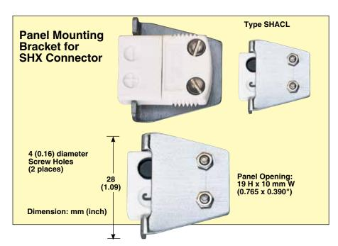
OMEGA® SHXJP panel jacks are designed for temperatures up to 538°C (1000°F), with SHX type subminiature ceramic connectors mounted to a steel plate. They are also available with unglazed connectors, type USHX, for applications where glazed connectors, would contaminate a vacuum system.
