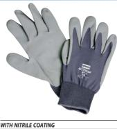
Seamless grey nylon liner to provide excellent fit and comfort, coated with textured grey Nitrile to give good grip also in oily applications. The good fit and grip allows the worker a high work efficiency e.g. handling small and oily objects.
