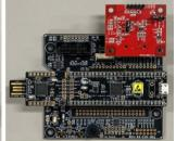
Ribbon cable connection Direct connection Figure 2. BU79100G-LA-EVK-001 connection
