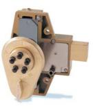
Light Commercial & Residential Lock All Metal Cast Front Force-proof Clutch Thumbturn Optional Manual Deadbolt or Auto Deadlocking Latch Option 35 to 54mm (1 3/8" to 2 1/8") Door Thickness
