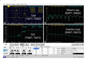
deskew ensures easy removal of fixture and probe effects. To get the best accuracy, mechanical calibration kits or ECal with DC option (i.e. N443xD or N469xD with Option 0DC) are recommended.
