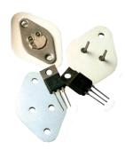
Tgard<sup>™</sup> 500 is a medium thermal performance insulator pad consisting of a ceramic filled, high temperature, silicone rubber coated on electrical grade fiberglass. Tgard<sup>™</sup> 500 has proven low thermal resistance after reliability and shows no delamination.
