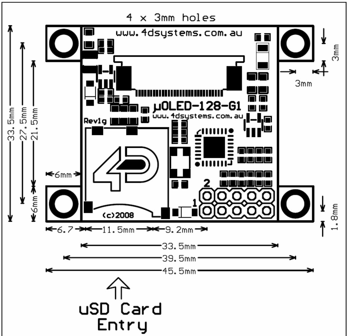
The module thickness is **6.3mm** (not including header pins)
