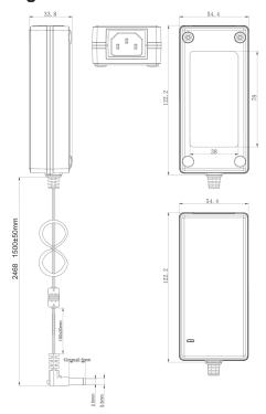
Dimensions : Millimetres Tolerance: ±0.5mm
