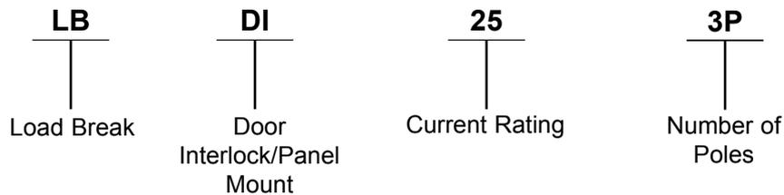
**Door Interlock/Panel Mount** : DI = Door Interlock and PM = Panel Mount.
