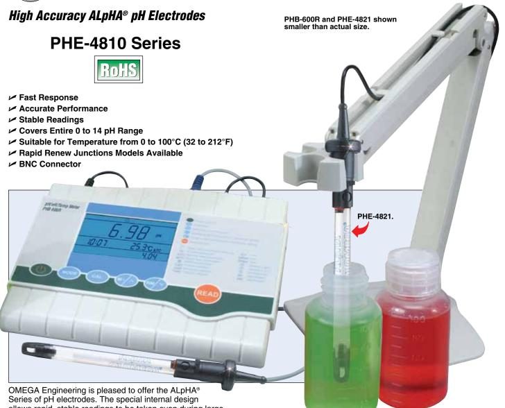
OMEGA Engineering is pleased to offer the ALpHA<sup>®</sup> Series of pH electrodes. The special internal design allows rapid, stable readings to be taken even during large temperature shifts. The double junction construction prevents silver ions from contacting the sample, eliminating reactions with heavy metals, sulfides, and proteins. ALpHA Series electrodes are available in a variety of styles to suit a wide range of applications.
