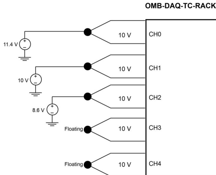
Figure 4. OMB-DAQ-TC-RACK common mode voltage connections example
