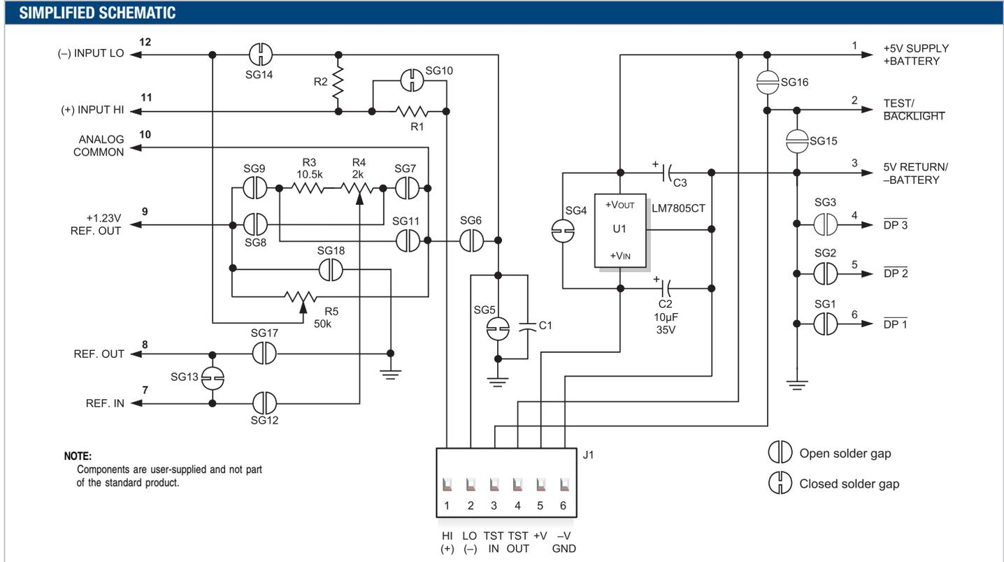
Figure 1. DMS-EB Schematic Diagram for DMS-30 Meters
