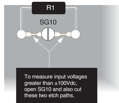
Figure 3. Installing R1
