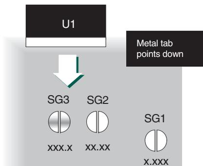
Figure 2. Installing U1
