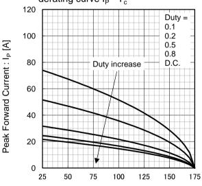
Fig.8\*4 Typical peak forward current derating curve I<sub>P</sub> - T<sub>c</sub> (Not guaranteed)
