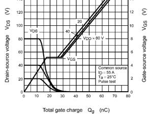
Fig. 8.10 Dynamic Input/Output Characteristics
