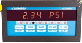
Alarms (Optional): Mechanical relay; 1 A @ 28 Vdc or 0.5 A @ 120 Vac, SPST, programmable as NO/NC, DC driver; 5 Vdc @ 50 mA; 1 alarm per channel
