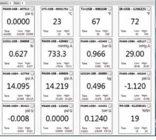
Channels Window – Display data from all of your sensors simultaneously. Each channel has configurable user alarms, three data filters, tare, resettable low/high indication, and sample rates ranging from 30 minutes to 1000 Hz.
