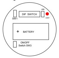
Switches 1, 2, 3 & 4 select the RF Network the IWPT will transmit on. The default network for both the IWPT transmitter and IWR receiver is network 1.
