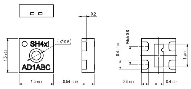
Figure 7 Dimensional drawing of SHT4xI-Digital including package tolerances (units mm).
