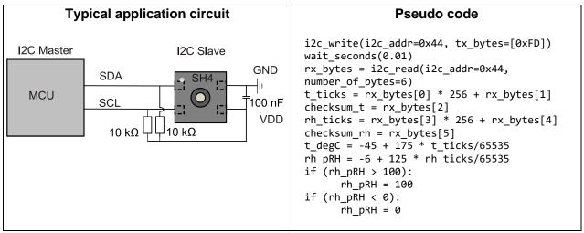
**Figure 1:** Typical application circuit (left) and pseudo code (right) for easy starting. For details on the signal cropping in the last four lines see **section 4.6**.
