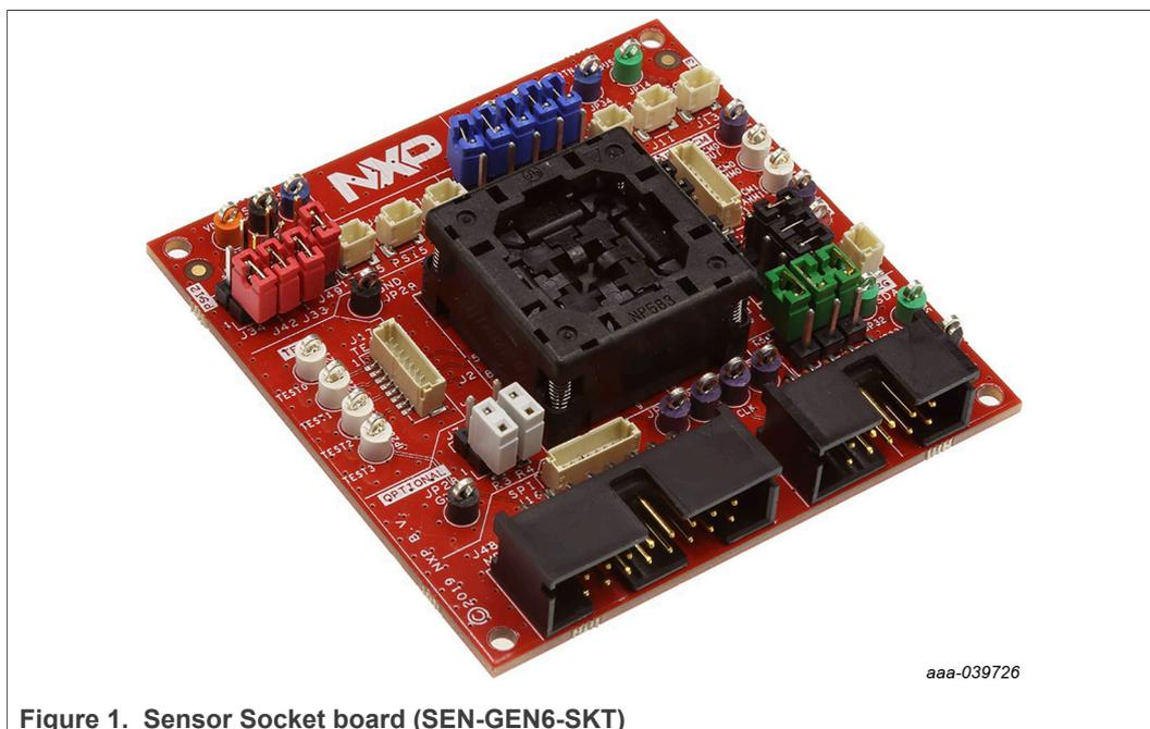
Figure 1. Sensor Socket board (SEN-GEN6-SKT)
