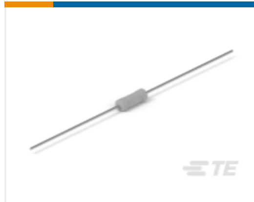
TE Part #7-1676123-9 1/2W SM M/OX 5% 1K5
