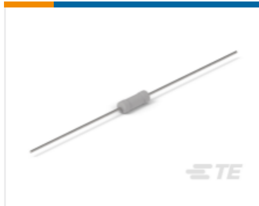
TE Part #7-1676123-7 1/2W SM M/OX 5% 1K2
