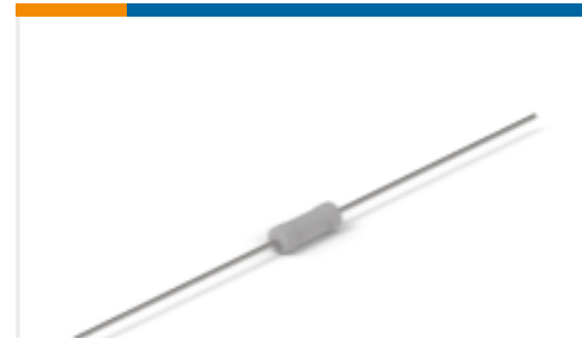
TE Part #7-1676123-7 1/2W SM M/OX 5% 1K2
