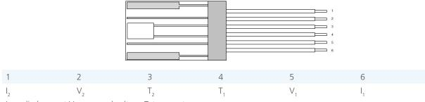
I: applied current V: measured voltage T: temperature sensor
