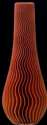
Smooth surface if model printed with international brass nozzle
