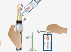
If there is still Resin left in the tube, discard the mixing nozzle S and replace the cap 4 for use with the next gland.
