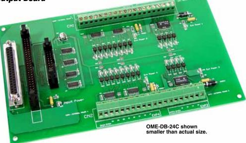
The transistor is energized by applying a 5 V signal to the appropriate input channel on the 50-pin connector, 20-pin flat cable connector or 37-pin D-sub connector. Twenty-four enunciator LED's, one for each transistor is activated.
