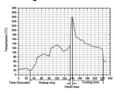
260°C ≤5 sec (Wave Soldering) 350°C ≤3 sec (Hand Soldering) Soldering Peak: 260°C - 10 sec (IEC 60068-20)
