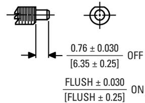
Note: Tolerance ± .005 [0.13] unless noted angles: ±5°. Dimensions in Brackets [ ] are millimeters.
