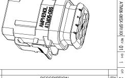
PLUG, KEYED, 8 SOCKET, STRAIN RELIEF, ATM SERIES DWG NO:
