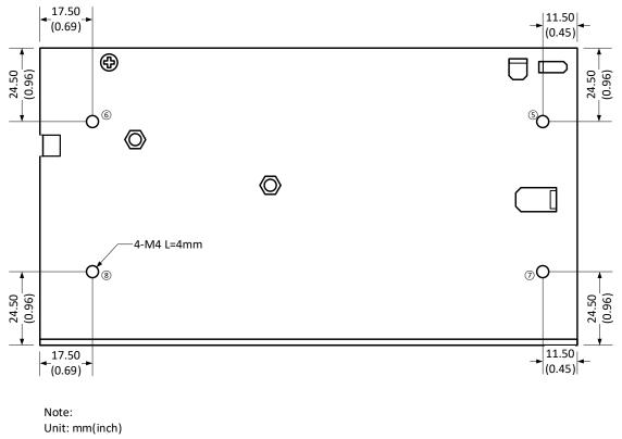
Unit: mm(inch) Wire gauge: 22-12AWG Screw terminal tightening torque: M3.5, 0.8N-m Mounting screw tightening torque: M4, 0.9N-m General tolerance:  $\pm 1.0(\pm 0.04)$ At least one of the 1 - 8 location must be connected to PE
