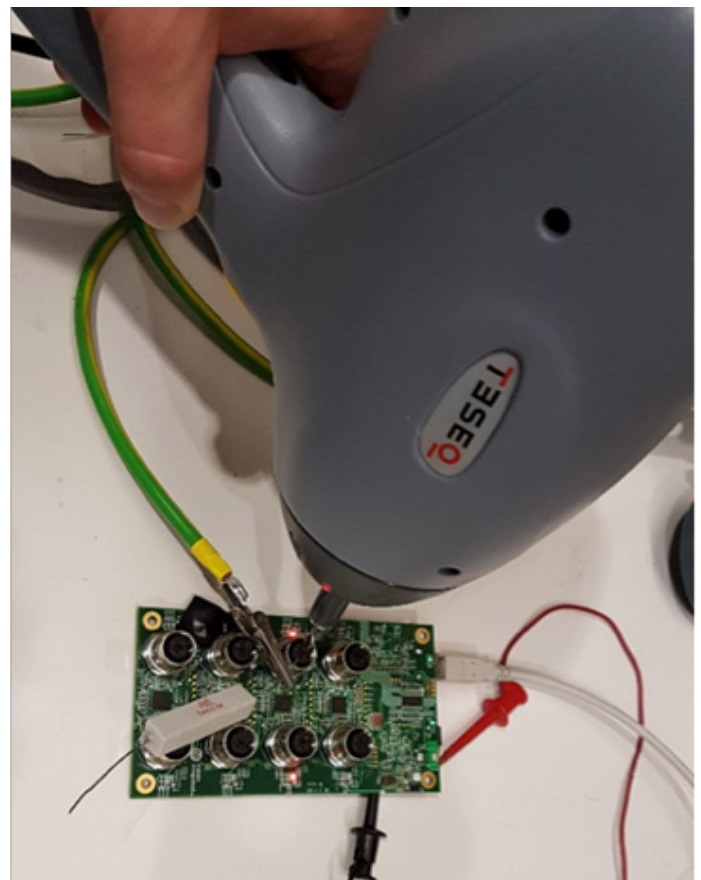
Figure 39. ESD Testing of MAX14819
