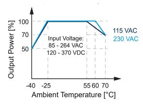
Figure 1. Temperature Derating Curve
