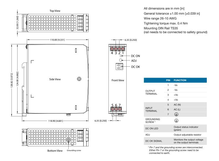
Figure 5. Mechanical Drawing
