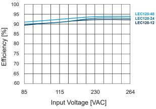
Figure 3. Efficiency vs Input Voltage Derating Curve (Full Load)
