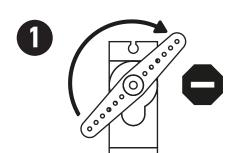
Connect a horn to the servo axle and gently rotate clockwise until it stops. Then rotate back an 1/8 turn.
