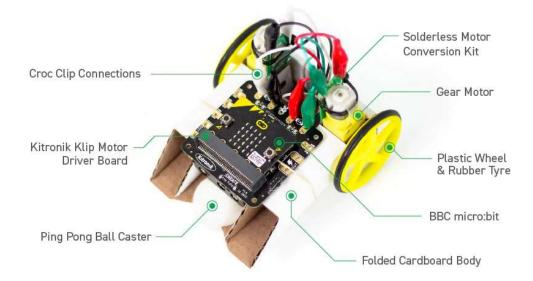
Our Simple Robotics Kit is an easy build, entry level, introduction to the exciting world of robotics. Step by step build and coding instructions are included.
