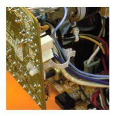
For retaining wires, cable, components or tubing away from panel or conductive chassis. Finger grip flanges can be easily locked or unlocked for revisions. Hand installed in pre-drilled hole.
