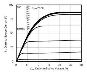
Fig. 1 - Typical Output Characteristics
