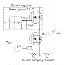
Fig. 18 - Gate Charge Test Circuit
