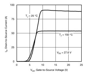
Fig. 3 - Typical Transfer Characteristics
