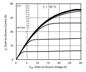
Fig. 2 - Typical Output Characteristics
