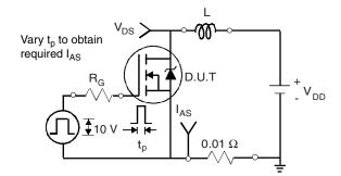
Fig. 15 - Unclamped Inductive Test Circuit
