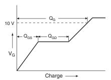
Fig. 17 - Basic Gate Charge Waveform
