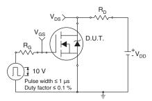
Fig. 13 - Switching Time Test Circuit
