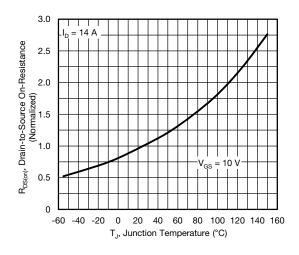
Fig. 4 - Normalized On-Resistance vs. Temperature
