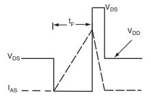
Fig. 16 - Unclamped Inductive Waveforms
