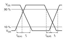
Fig. 14 - Switching Time Waveforms
