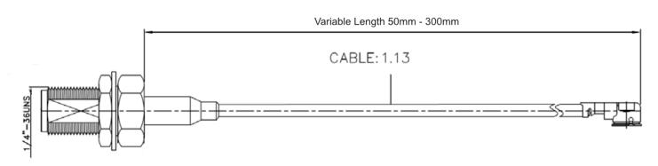
SMA Female Bulkhead Connector to MMCX Connector example drawing
