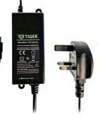
The Tiger Power TP1016-DIM is a power supply supplied complete with a PWM dial dimmer switch which can be used to adjust the brightness level of any 12V constant voltage LED lighting, including LED strip, up to 2A (24W) max. Its supplied complete with integral UK mains lead. The screw holes which are integral to the plastic enclosure enable the power supply to be fixed down. Approved to latest safety and efficiency standards
