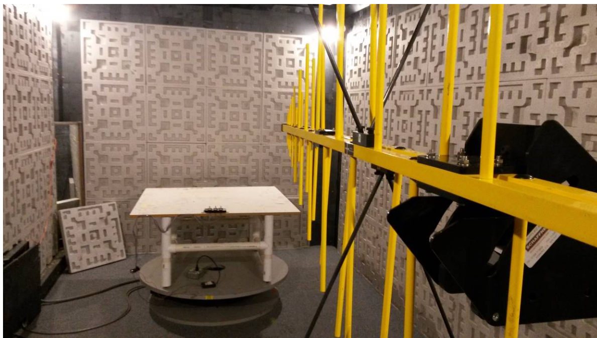
Figure 11 – Radiated Emissions Test Setup
