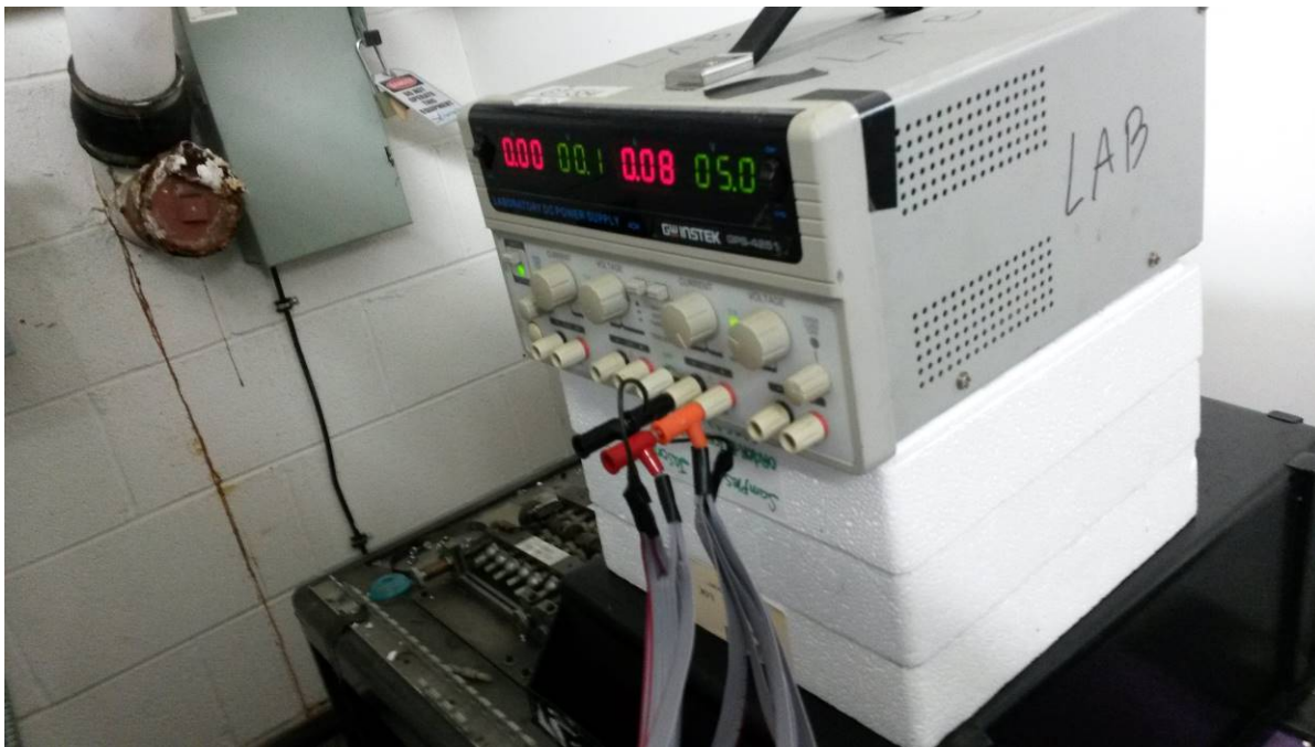
Figure 1 – 85/85 Humidity Electrical Test Setup
